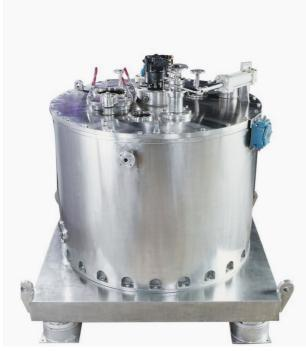
A Top-Driven Bottom Discharge Centrifuge is a vertical batch-type centrifuge where the drive motor is located at the top and the solids are discharged from the bottom using an automatic scraper or peeler mechanism.
