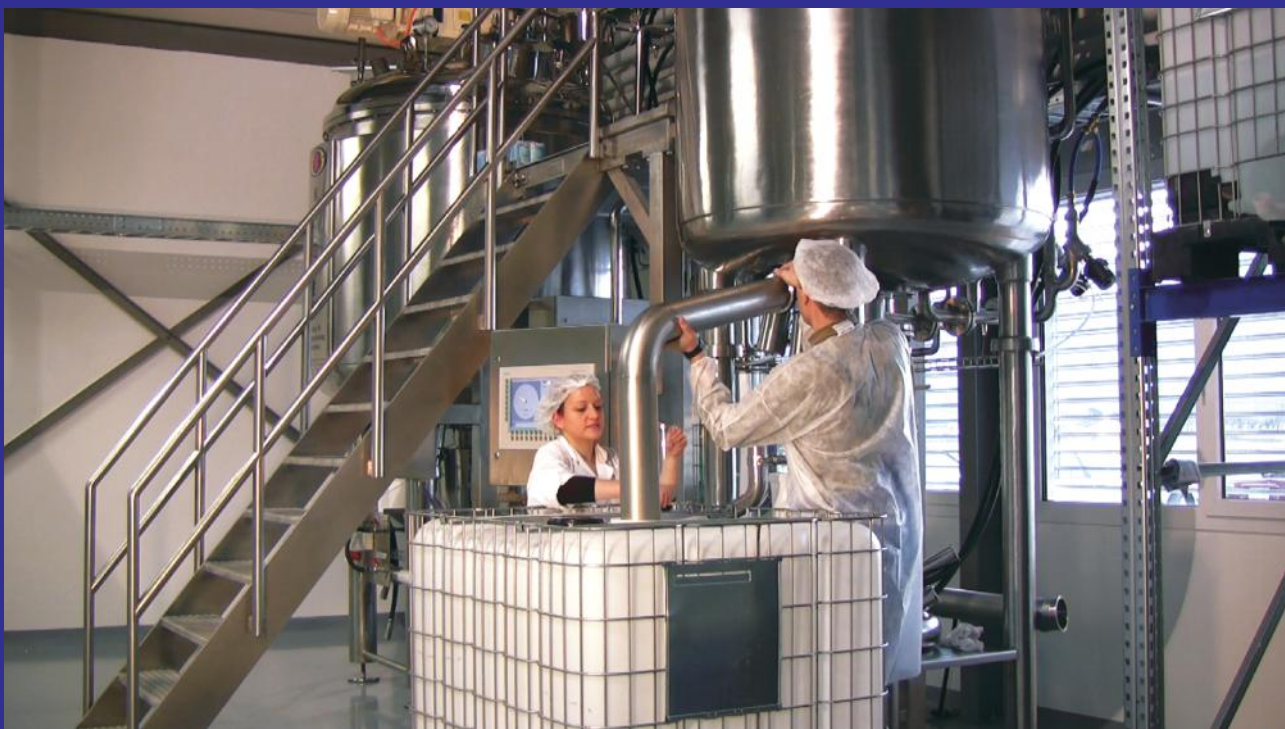
Discharge of a 1000 liter vessel by gravity and/or pressure
