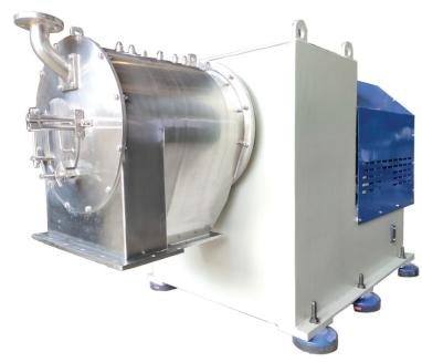
A pusher centrifuge is a horizontal, continuous machine for separating free-draining crystalline or fibrous slurries, pushing solids to discharge as liquid filters through the basket walls.
