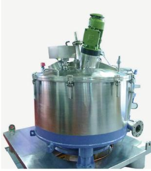
A pull-action vertical batch centrifuge discharges solids from the basket bottom in two steps. First, at reduced speed, a scraper peels the cake from the filter cloth and pushes it out. Then, a hydraulic bottom ring pulls the filter bag downward, shaking off residual heel and leaving the basket nearly clean.
