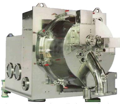
A pharmaceutical peeler is a horizontal batch type centrifuge designed for sterile, GMP-compliant API and fine powder production, featuring full jacket opening, electropolishing, and high containment. A mechanical blade scrapes and discharges the solids automatically.
