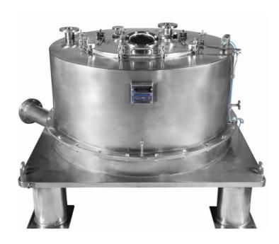
A Manual Top Discharge (MTD) centrifuge is a vertical batch-type centrifuge where solids are manually scooped from the top of the basket after the separation process.
