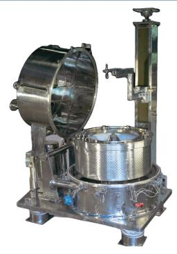
An Instant Top Discharge Centrifuge (ITD) is a vertical batch-type centrifuge that offers semi-automatic discharge of solids from the top using a bag lifting device (BLD), significantly improving upon traditional manual top discharge centrifuges.
