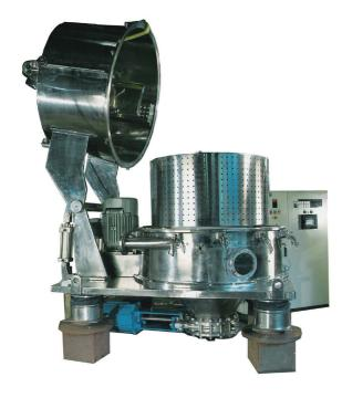
A Bottom-Driven Bottom Discharge (BDBD) centrifuge is a vertical batchtype machine that uses an automatic scraper or plough to discharge solids from the bottom. The drive system sits below the basket, keeping the top area clear.
