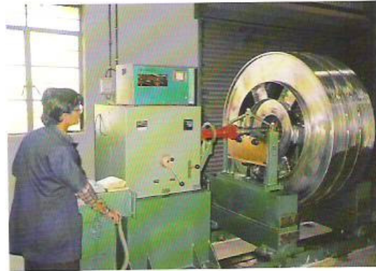
Bottom Discharge Centrifuge basket being dynamically balanced on our Computerised Dynamic Balancing Machine
